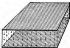
FIG. 35.—Diagrammatic Section of a Charged Condenser Formed by Two Parallel Plates, Showing the Distribution of Electric Flux in the Insulator Between Them.
